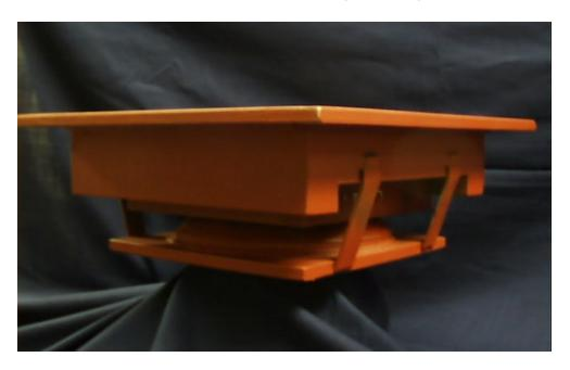
The **ULR-SA** (Uplift Restraint Spherical) with guide system eliminates the need to design elaborate and expensive structural arrangements to control directional movement by having the guide system built into the bearing.
